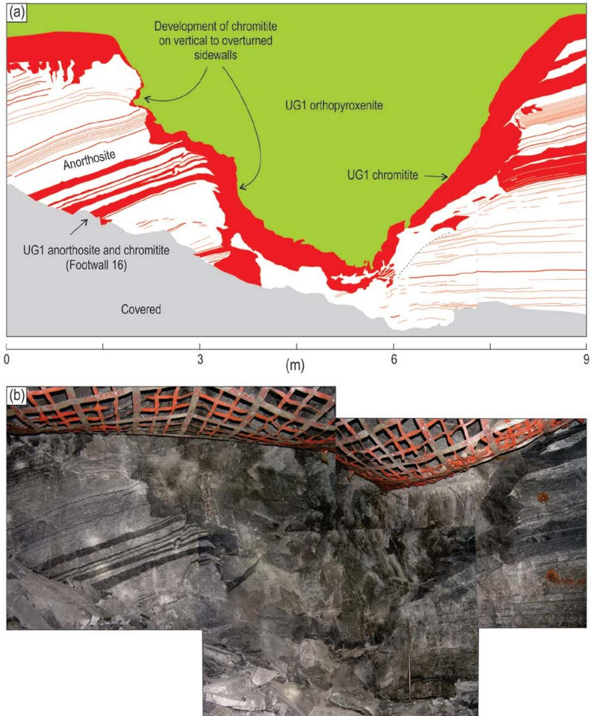
Fig. 1. Sketch (a) and photograph (b) of an oblique cross-section showing UG1 chromitite draping over steeply-inclined to overhanging walls of a pothole. Note crosscutting relationships of the UG1 chromitite with interlayered anorthosite and chromitite in the footwall rocks and disrupted layering on the right side of a pothole. Level 15, Shaft 10 of the Impala Platinum Mine, Western Bushveld.
